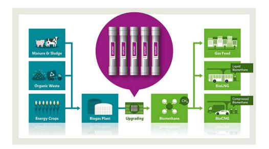
**Image capture:** Biogas is produced by fermentation of biomass. It can be easily and efficiently upgraded to high-purity biomethane by means of SEPURAN<sup>®</sup> Green membranes and used decentralized as a climate-friendly energy source. (©Evonik).
